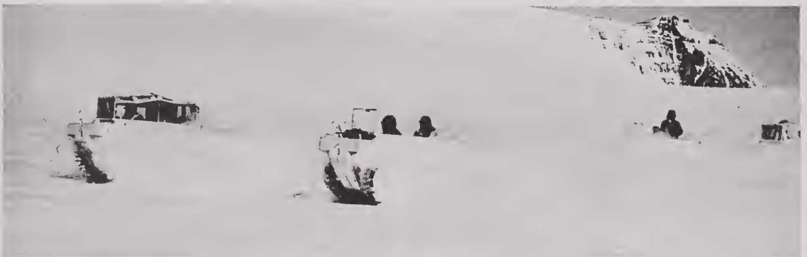
FIGURE 36. Pilot models of T-15 Weasel outdistancing skiers in tactical test on Columbia Ice Fields. Even with the advantage of an 1,800-foot schuss from high ridge shown at upper right, skiers were beaten by 41 minutes over 2.9-mile test course.
